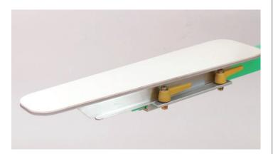
Tapered sleeve platens allow versatility when printing standard long-sleeve garments and newer styles that are tapered at the wrist. *Photo courtesy of Action Engineering*.
