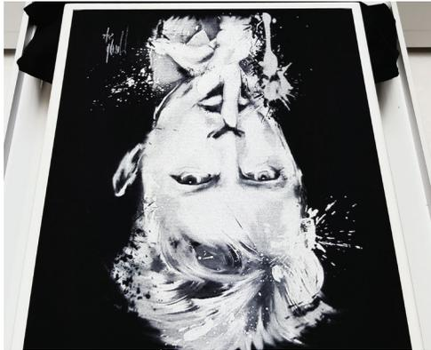
**STEP 5** The first pass on a dark shirt is the white underbase, which is created by the software.
