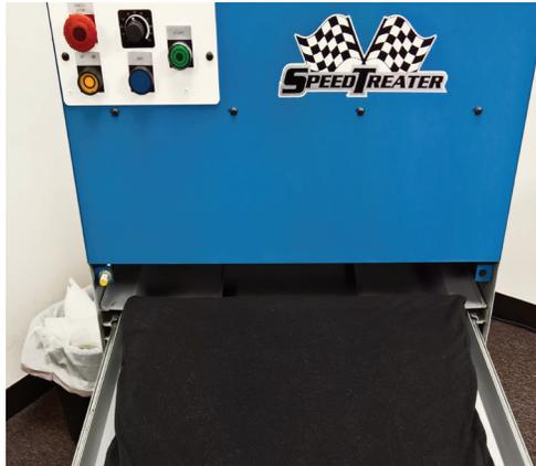
**STEP 3** The heat press is used to dry the pretreatment solution on the shirt before printing.
