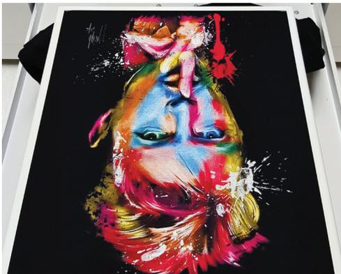
**STEP 6** Here is the garment after the underbase print and the CMYK pass of color to complete the image.
