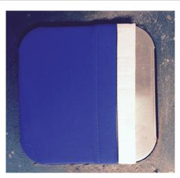
A straightedge piece of cardboard is adhered to the platen for aligning the fabric and to add off-contact support for the bra hem.
