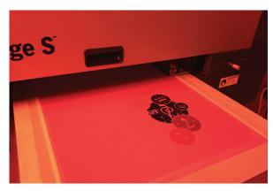
Screens are imaged with a direct-toscreen (DTS) imaging system. MINIMAL OFF CONTACT SETTING
