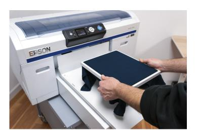
The garment is being loaded on the Epson F2000 10" x 12" shirt platen.
