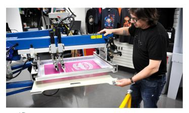
Register the four-color print on the M&R Sportsman using the M&R Tri-Loc platen to align all screens.
