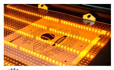
The films were pre-aligned on each screen with the M&R Tri-Loc system, exposed for 9 seconds on the M&R Starlight LED exposure unit and washed out.
