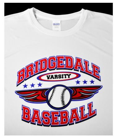
With the squeegee angle set at 15 degrees on the white performance garments, adjust the squeegee pressure at 40 PSI with medium squeegee speed. Print wet-on-wet without flashing.
