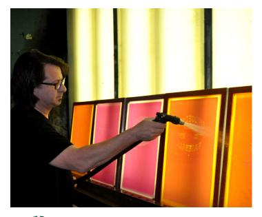
Wash out the image on a back-lit washout booth with a water.
