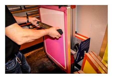
The screens were coated with KIWO Multi-Tex high-solids emulsion and a "one-on-one" coating technique with the scoop coater's dull side.
